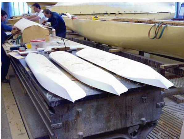
Fig. 7. Wedges applied to the models in order to obtain the correct floating position
